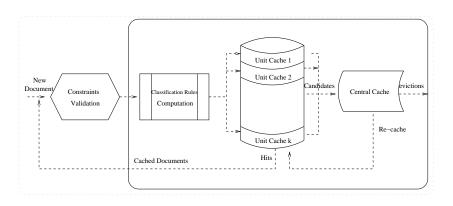
Fig. 1. Framework of constructed replacement policies
