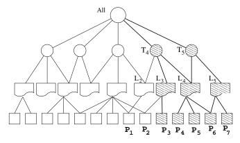
Fig. 3. Cache replacement based on the hierarchical model.
